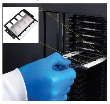
Figure 3. PhenoImager HT slide carrier and slide hotel.
