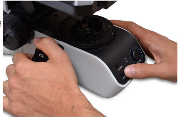
Figure 15. The Mantra 'Snap' button to take pictures is located on the handgrip on the left side of the Mantra instrument base. In the picture above, the Snap button is located under the user's left thumb. The Objective rocker switch to change objectives is located under the user's right thumb.
