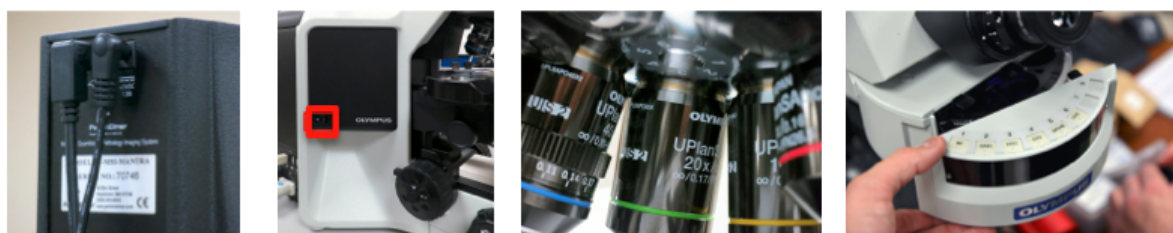
Figure 3. Power and USB cables plugged into the back of the Mantra imaging module (far left); the location of the Mantra Power switch outlined in red (middle left); objectives in their numbered turret positions (middle right); and epi-fluorescence filter cubes in their designated, numbered locations (far right).
