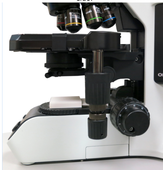
Figure 56. The right side of the Mantra instrument shown here with the knob for focus adjustment on the right. To the left of the knob are the stage controller knobs for X and Y axis control of the specimen under the objectives.
