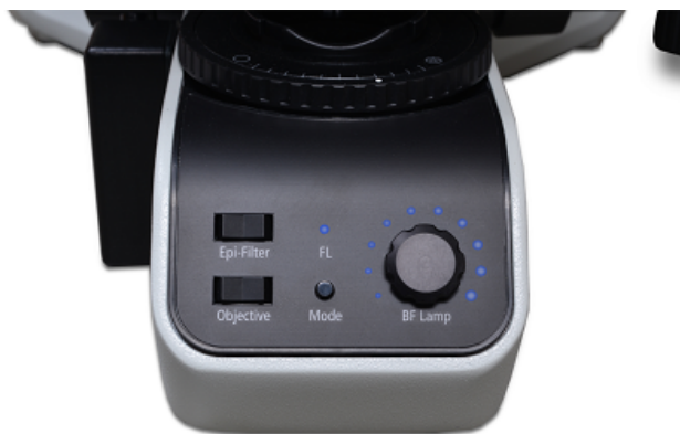
Figure 32. You can use the Epi-Filter rocker switch to select the epi-fluorescence filter that you wish to use, and the Objective rocker switch to select the objective you want to use. In fluorescence mode, the blue light above the FL (fluorescence) label is lit. The BF Lamp knob for setting the brightfield illumination level is deactivated when you are in fluorescence mode.
