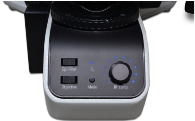
Figure 12. You can use the Objective rocker switch to select the objective you want. In brightfield mode, the blue light above the FL (fluorescence) label remains off and the Epi-Filter switch is deactivated. You can set the illumination level that is comfortable for you through the eyepieces using the BF Lamp knob on the right.
