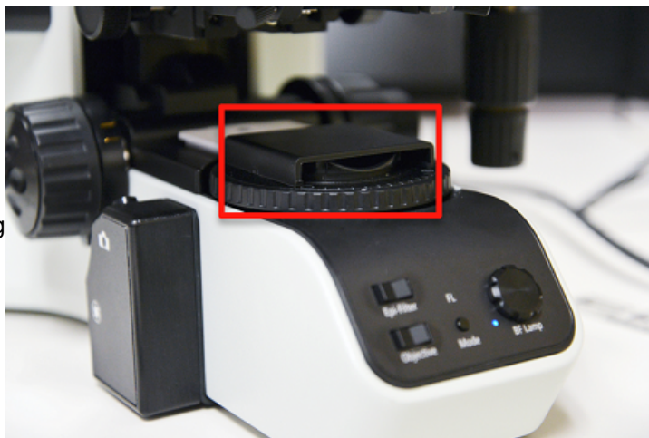
Figure 25. The Beam Block (the plastic cover shown in the red box) slides over the brightfield illuminator when you are using the Mantra system to take fluorescence image. The Mantra Snap program will prompt you to slide it into or out of place when necessary.
