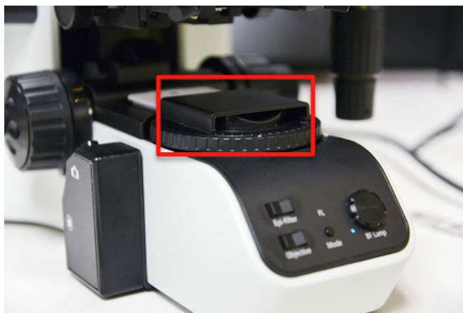
Figure 9. The Beam Block (the plastic cover shown in the red box) slides over the brightfield illuminator when you are using the Mantra system to take fluorescence image. The Mantra Snap program will prompt you to slide it into or out of place when necessary.
