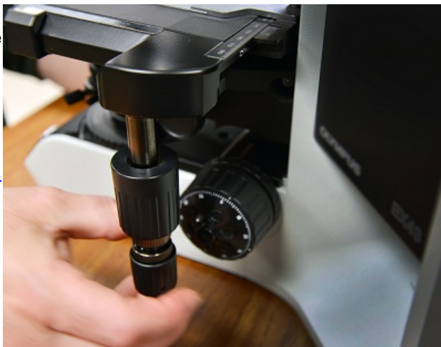
Figure 13. Use the Stage Control knob located by default on the right side of the Mantra instrument to move the microscope stage along the X- and Y-axes.
