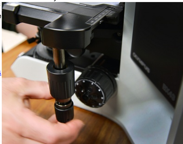
Figure 33. Use the Stage Control knob located by default on the right side of the Mantra instrument to move the microscope stage along the X- and Y-axes.
