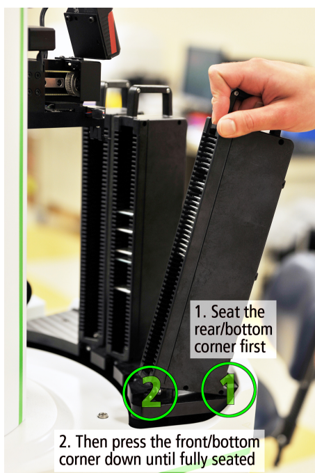
Figure 9. Mounting Slide Cassettes to the Slide Loader
